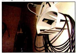
Fig. 2: Garden hose hangers are good for hanging coaxial test cables.
