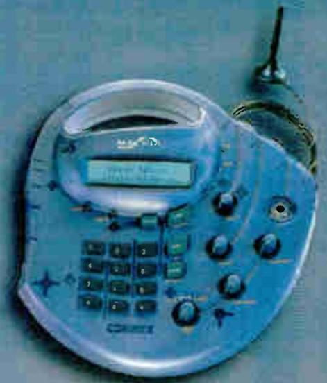
Delivering the sound of the summit to listeners around the world is as simple as pressing a button. The Comrex Matrix, equipped with our optional GSM Module, combines an integrated mobile phone and an advanced Comrex codec to deliver broadcast quality 7kHz audio over standard cellular connections (15kHz over POTS).
