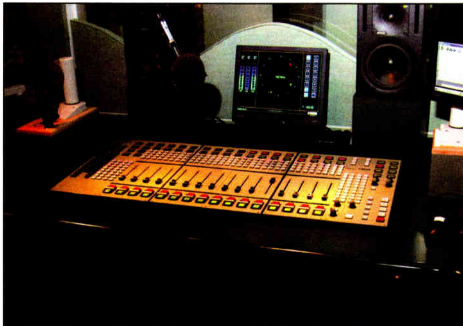
A 16-fader Klotz DC II Digital Mixing Console is located in the rear of Performance Studio 1, for primary on-air/production duties.
