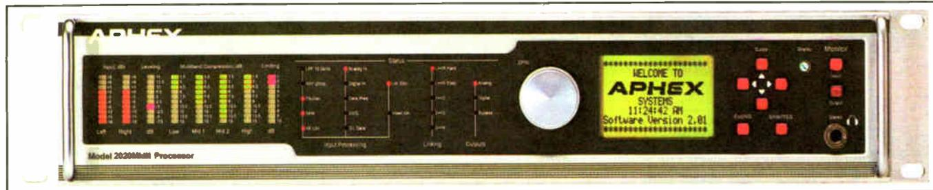
The multi-functional 2020 MkIII features a wave-dependent compressor and sticky leveler.
