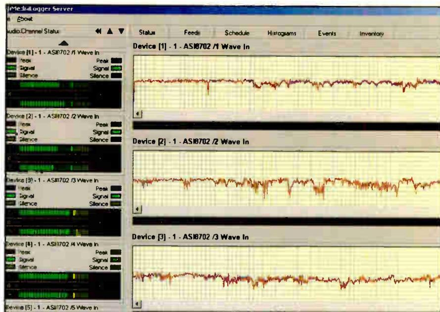
iMediaLogger records up to 12 stereo/mono audio sources simultaneously, and supports multiple compression formats.
