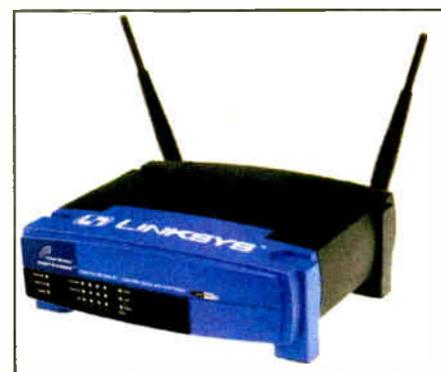
The author used a Linksys BEFW11S4 EtherFast Wireless AP + Cable/DSL Router w/4-Port Switch. It connects a wireless network to a high-speed broadband Net connection and a 10/100 Fast Ethernet backbone.
