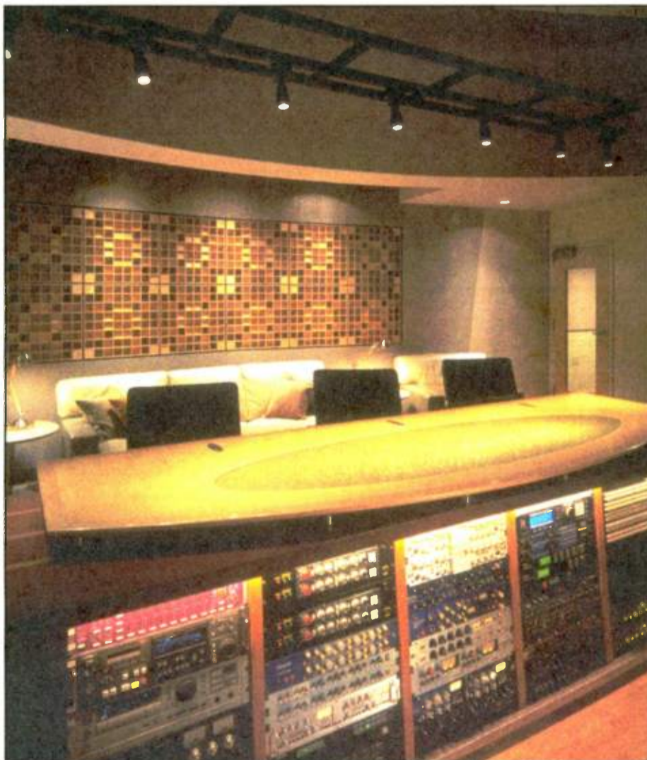
Fig. 7: Sound Diffusion Combined With Absorption
