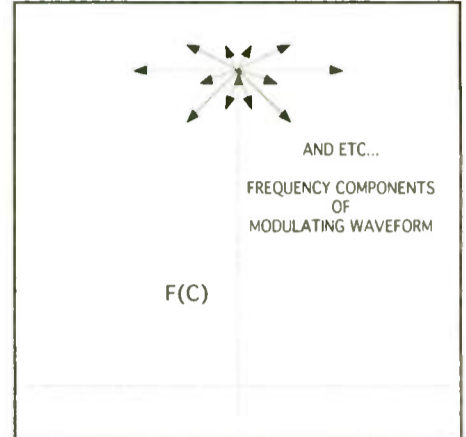
Fig. 5: AM Complex Modulation (Vector Representation)
