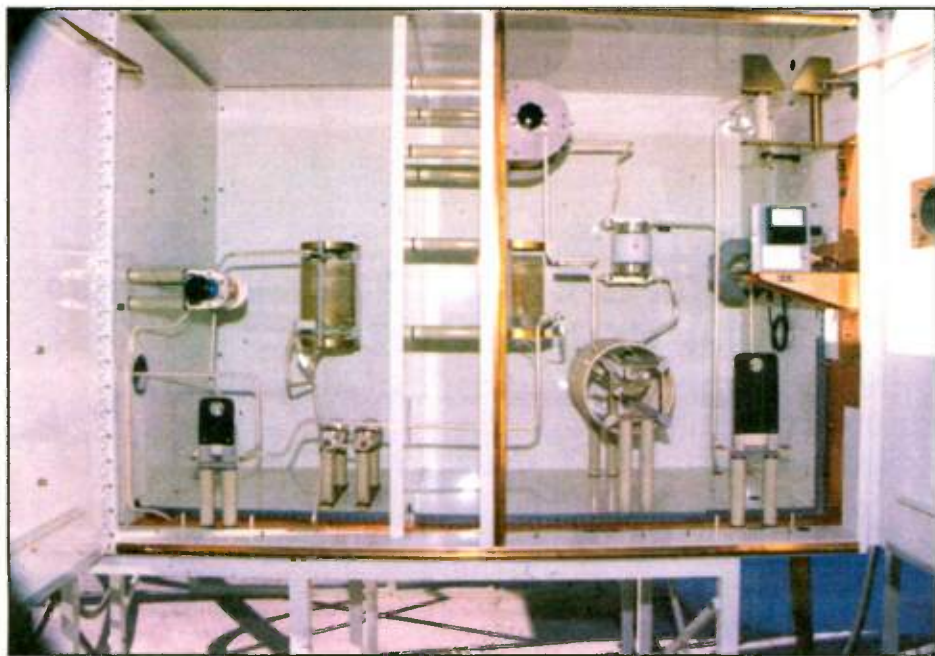
Fig. 6: Avoid long parallel tubing runs where possible.
