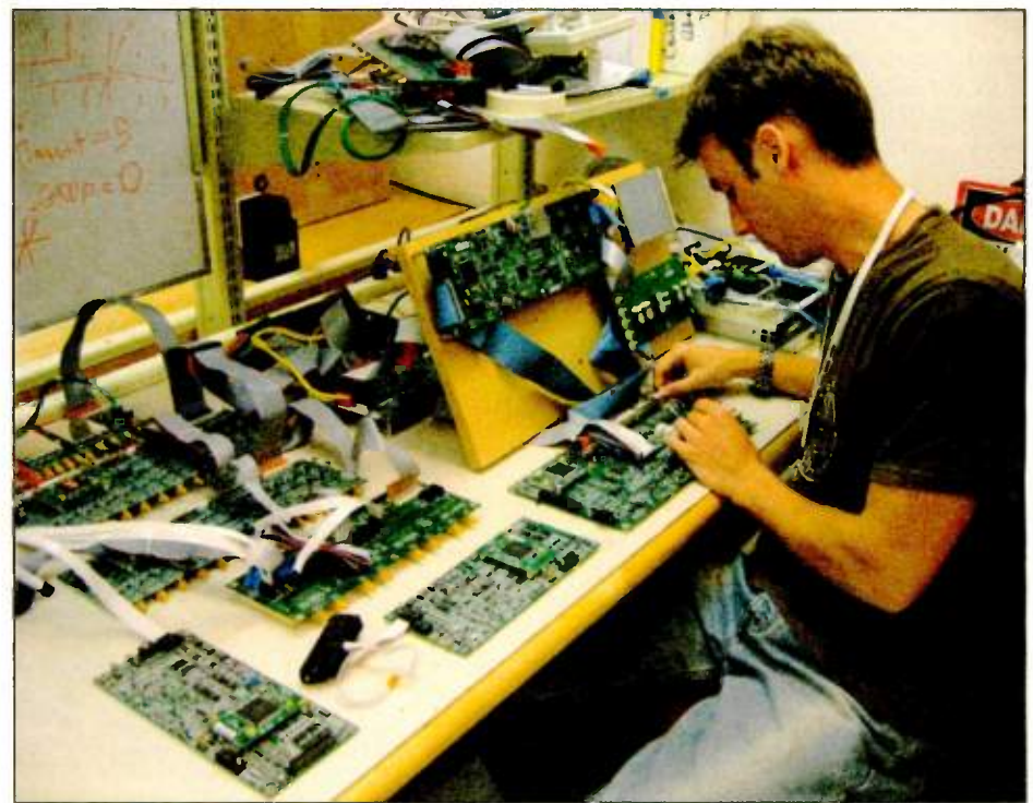
Fig. 4: Distributed Transmitter Control Architecture Breadboard That Is Re-used Across Product Lines
