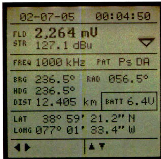
Fig. 3: Front-panel display of the FIM-4100
