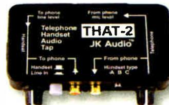
**THAT-2** Simple, convenient, professional. All JK Audio handset interfaces adapt to electret, dynamic, and carbon telephone handsets.
