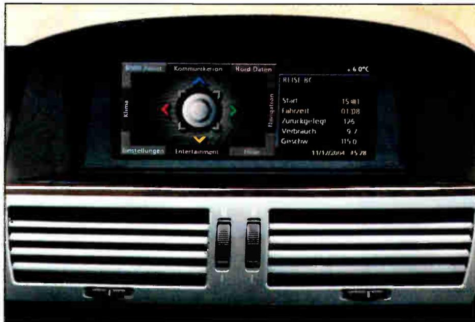
The left, rectangular window displays the main menu, a graphic display of the BMW controller with colored arrows pointing to eight available menus. The right, square window is displaying date, time, temperature and onboard (trip) computer data.
