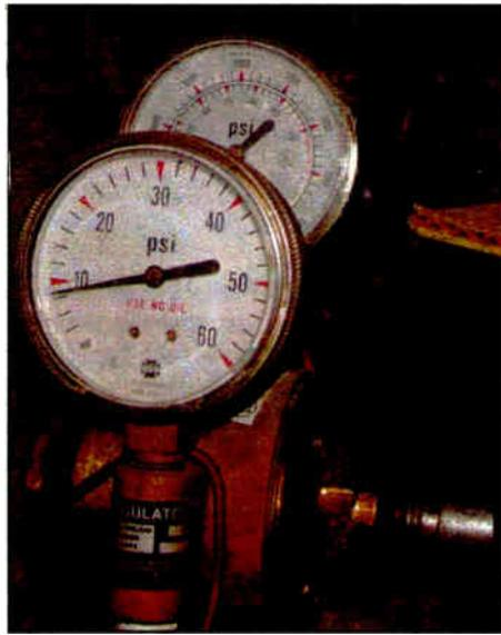
Fig. 4: Monitor line air pressure; it should never read zero.
