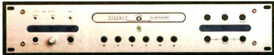
The Plan B Deluxe is a 2 RU box that senses audio loss prior to processing and can replace regular program audio with a backup source — basically a radio station in a box. In its loaded configuration, you have a ton of options on how you want to use it.
