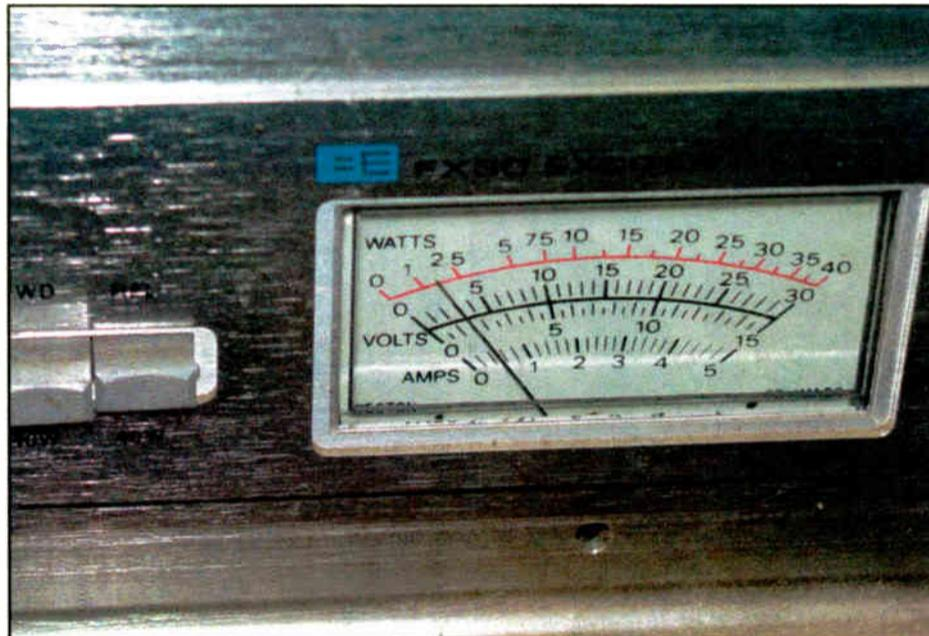
Fig. 2: Keep reflected power as close to zero as possible. This reading is less than desirable.
