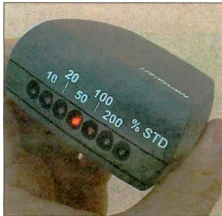
Fig. 6: The Nardalert personal monitor detects RF emissions and weights the field intensities in accordance with the FCC MPE.
