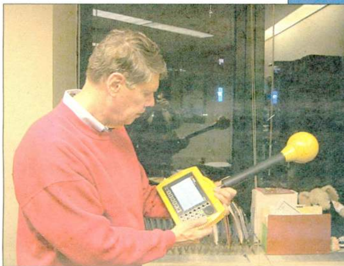
Fig. 2: Richard Tell uses the Narda SRM-3000 portable spectrum analyzer and isotropic antenna to document RF field level in a building adjacent to the 4TS site.
