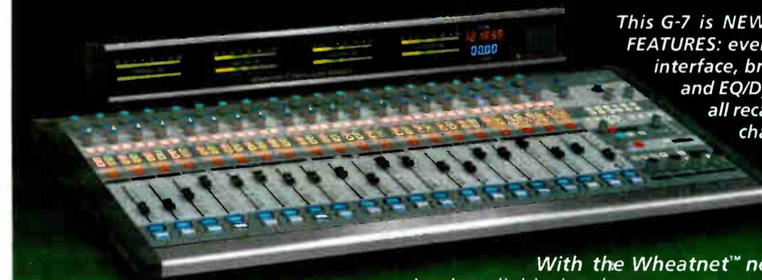
This G-7 is NEW and LOADED with FEATURES: event recall, automation interface, bright source displays, and EQ/Dynamics and panning, all recallable on EVERY input channel for production or mic processing—the list goes on.
