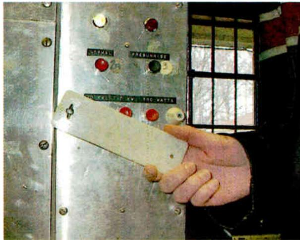
Fig. 1: Harry Bingaman used parts from his junk box to make this protective switch cover.
