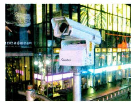
Already in use on several paths in RF-crowded New York City, including between the Empire State Building and lower Manhattan, RF~IPMax uses 5.8 GHz spread-spectrum transmission to provide up to 49 Mbps of Ethernet throughput along paths up to 50 miles line-of-
