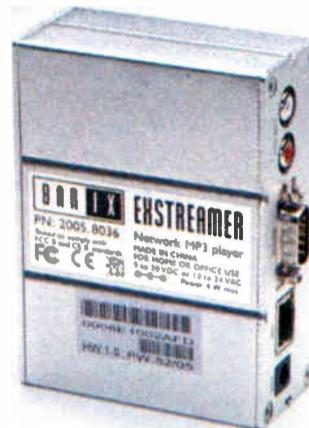
General Manager Mike Afflerbach connected one Instreamer, based at the studio, to the output of an existing EAS system. Once initiated, the EAS system sends audio to the Instreamer, which relays the audio to the Exstreamer devices located at the various transmitter sites. The priority port in each Exstreamer sends the EAS signal to the transmitters for broadcast over the air, and the EAS Instreamer shuts down following the EAS broadcast.
