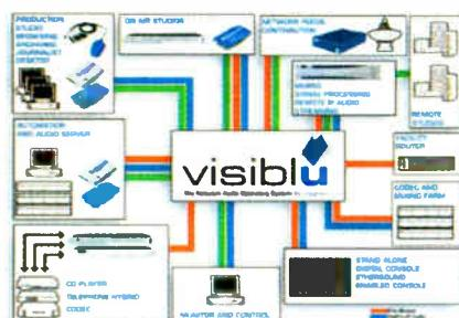
company says it unifies the EtherSound low-latency Ethernet protocol with RTP/UDP IP audio streams in an engine that runs under both Windows and Linux.
