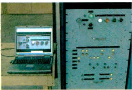
Access to the controller Web port will require a user-defined password. Utilizing a software-driven programmable logic controller to emulate standard relay logic, the controller will require less rack space than a standard relay logic controller.
