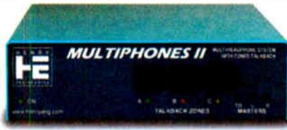
The unit supports up to 12 Guest Pod listening stations, and includes a 3 Zone Talkback feature, which allows talkback to individual or groups of Guest Pod users. The Multiphones system provides each headphone listener with an individual jack, amplifier and volume control, which are interconnected by Cat-5 cabling.
