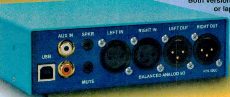
Both versions feature easy USB interface to any PC or laptop. Balanced analog inputs and outputs at professional levels are on XLR connectors. The Speaker output can be used for monitoring, with muting via any GPI closure.
