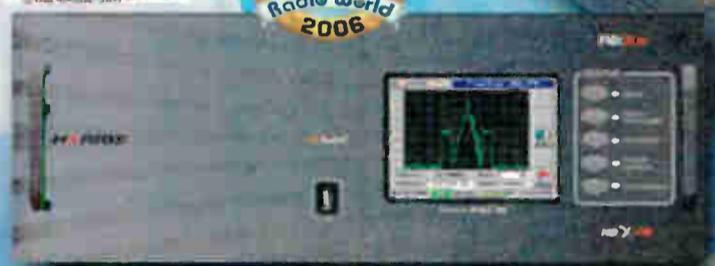
FlexStar HDx exciter—the gold-standard for FM and FM-HD exciters, featuring RTAC (Real Time Adaptive Correction for best mask compliance) and Exgine, the latest iBiquity platform in HD Radio.
