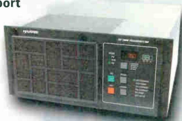
ZX1000, 1 kW tri-mode FM/FM-HD or digital only transmitter. FM transmitters available from 250 W to 70 kW, in analog or HD Radio.
