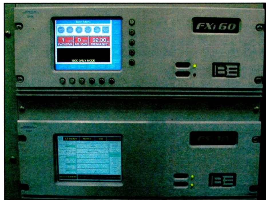
Fig. 2: Digital excitors and HD generators with internal CD-ROM drives in them initially seemed out of place at transmitter sites — and they still do!
