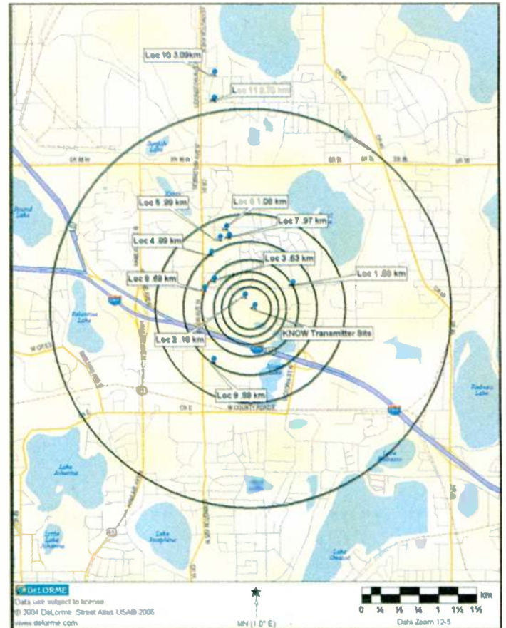
Fig. 7: Map showing predicted locations of signal nulls from the KNOW main antenna from vertical plane plot.
