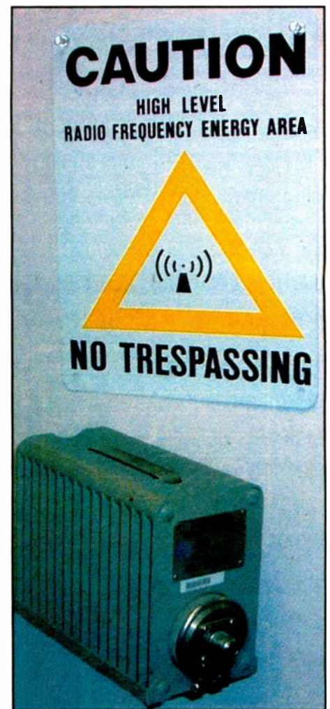
Fig. 3: This load may be a bit undersized for full-power Class B or C high-level reject load applications.
