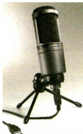
Audio-Technica introduced the AT2020 USB cardioid condenser microphone, based on its AT2020 and featuring a low-mass diaphragm.
