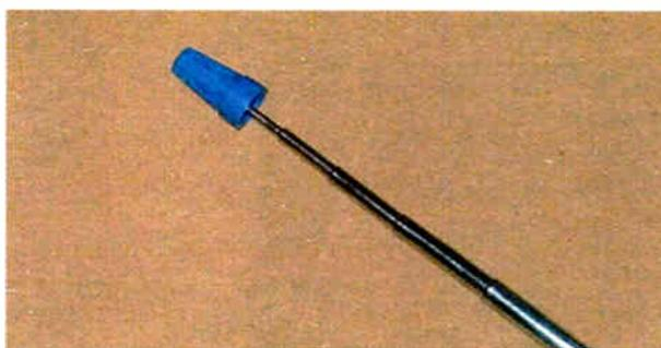
Fig. 2: This wire nut on the end of a broken antenna prevents the end from collapsing.
