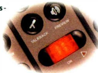
long-life components that they actually built a mechanical "finger" to test switches! Some supposedly "long life" switches failed after just 100,000 activations; when they found the switches used in Element, they shut off the machine after **2 million operations** and declared a winner. (The losers got all-expense-paid vacations to the landfill.)
