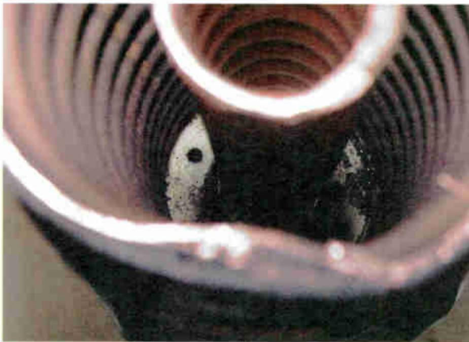
Fig. 2: Soot is nearly impossible to clean from flexible lines.
