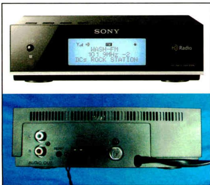
The two-pronged power cord is captive. The other connections on the rear panel are a pair of RCA pin jacks for audio out, an F female panel jack for antenna and a pair of press-release wire posts for the external balanced AM loop antenna.
