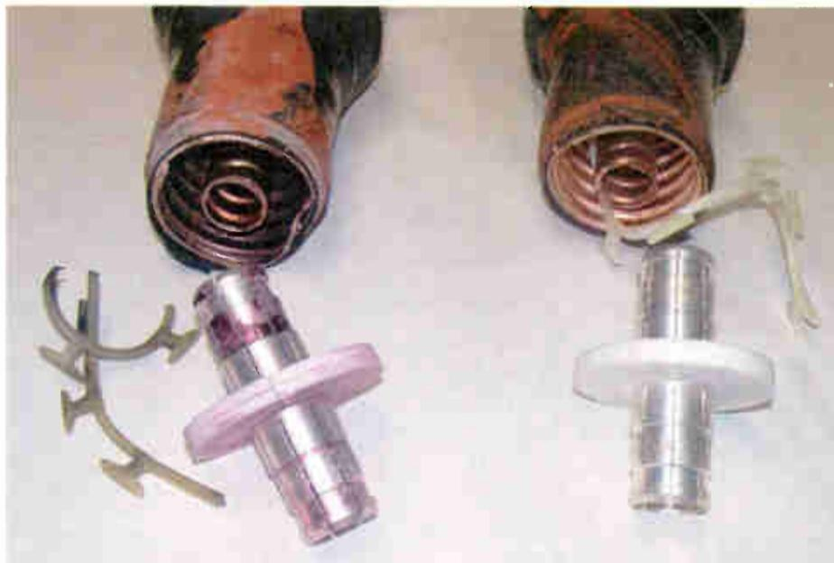
Fig. 1: This flashover damage to transmission line was caused by a hunter.
