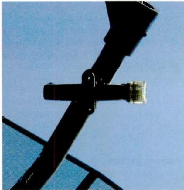
Fig. 1: Mount a waterproof laser pointer to your satellite dish to verify alignment.
