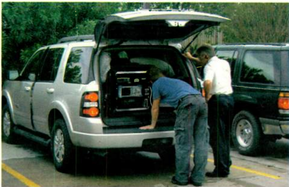
Field agents Paul Coburn, left, and Loyd Perry use a spectrum analyzer in Louisiana as part of the FCC's Project Roll Call system, which measures broadcast activity within a 30-mile radius before and after a hurricane.
