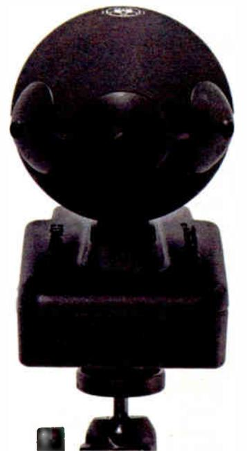
For adding surround to any studio, field recording and ENG application, the PortaMic Pro comes with a Dolby Laboratories' Dolby Pro Logic II encoder. The mic's six audio channels thus can be encoded down to two, so it can be recorded to any broadcast camera or stereo recording device. The PortaMic Pro is able to supply this encoding in a one-inch high encoder, providing a surround recording while offering an uninterrupted sightline when connected to a camera.
