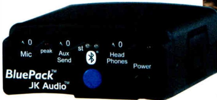
The potentiometers are countersunk nicely to protect them from accidental movement. They also have a solid resistance that provides the user with assurance that the selected level will not inadvertently be altered. Also, in this regard, the numbered indices on the pots let the user remember the preferred settings.
