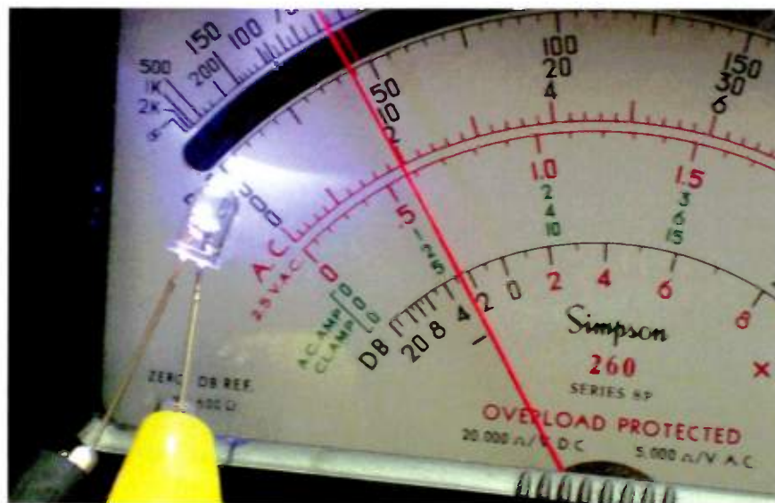
Fig. 2: The trusty old Simpson meter is used to check operating parameters of the LED before installation.
