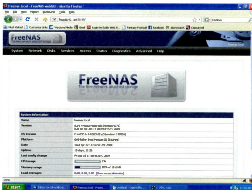
The main configuration screen for FreeNAS
