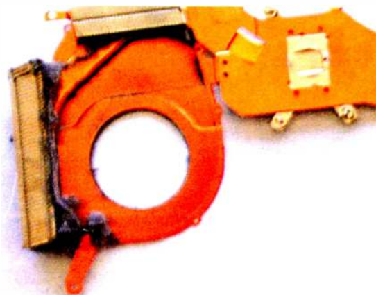
Fig. 2: This laptop suffered a complete processor failure due to dust on the heat sink.
