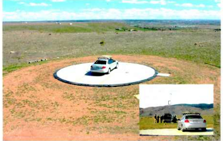
Fig. 6: The ground plane antenna undergoing calibration on the 30-foot turntable at Table Mountain Test Range, north of Boulder. The horizontal pattern uniformity on the vehicle was performed by rotating the entire vehicle, which contained a reference signal generator, and measuring test signals from a calibrated receive antenna near the measurement van, visible in the background.
