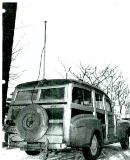
Top: Fig. 1: A 1948 Ford 'woody' station wagon used for the antenna proof of WJZ(TV), Channel 4, Detroit, taken in the winter of 1950-51.
