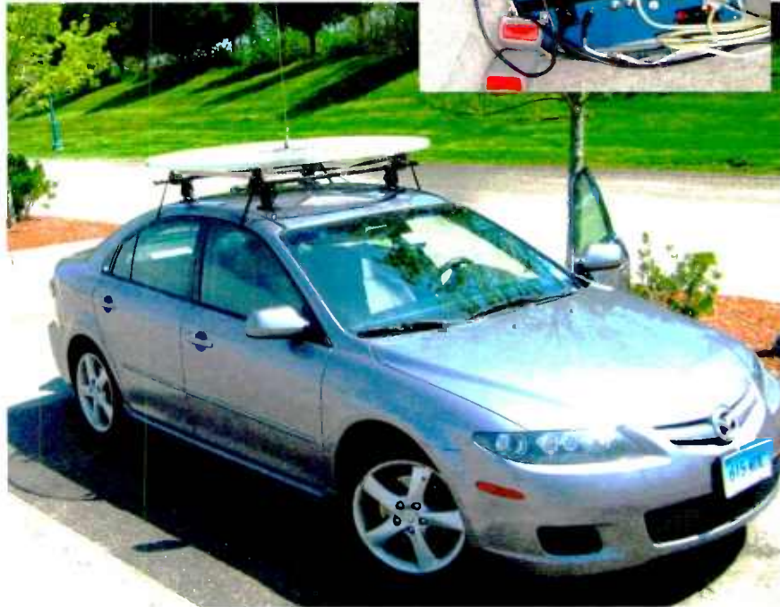
Fig. 4: A rental car equipped with NPR Labs' calibrated ground plane measurement antenna, taking signal and interference measurements near Brush, Colo. Inset: A backseat view of the Field Test Unit, configured for three-signal field strength collection (lower unit) plus HD Radio tracking and data logging (upper unit).
