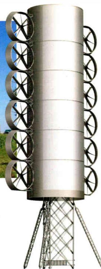
Fig. 2 (right): Arist's conception of a six-level, 300 kW turbine.
