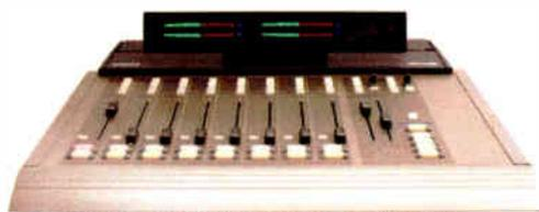
Called the Oasis, it is an 8-to-12-channel board. In a bow to digital reality it does offer digital outputs and, as Harris notes in a press release, a digital migration path.
