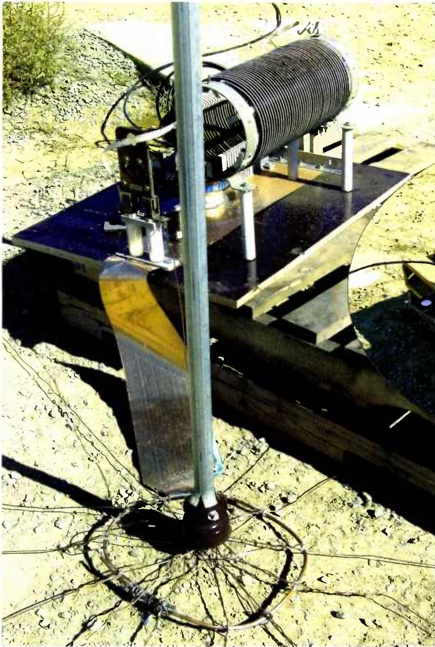
Left: Antenna base, bell insulator, ground ring/radials and tuning network.
