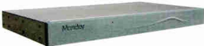
Rincon operates in a number of station topologies, point-to-point unidirectional, point-to-point bidirectional, and point-to-multipoint multicast.
