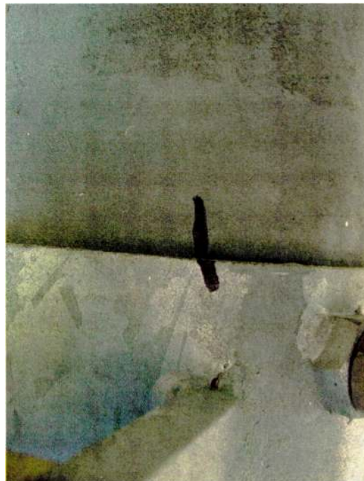
Fig. 3: Mark the rotating pedestal.
