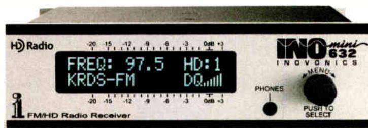
The \$850 box is described as a professional-grade FM and FM/HD-Radio receiver for off-air monitoring at stations multicasting FM and HD Radio aux channels 1-8. Analog FM and HD Radio digital programs are accompanied by digitized text and "housekeeping" data. FM RDS and HD Radio PAD are shown on the front LCD display, along with read-outs of signal quality information.
