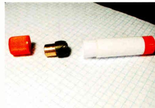
Fig. 6: Add a short piece of copper tubing to the glue well (black plastic) of the movable piston.
