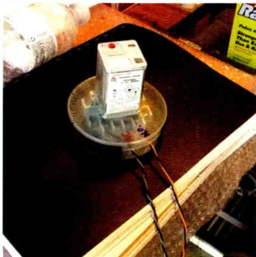
Fig. 1: An inexpensive alternative to a project box.
