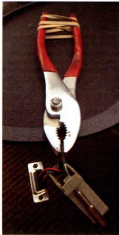
Fig. 1: A few rubber bands turn a pair of pliers into a simple third hand.
