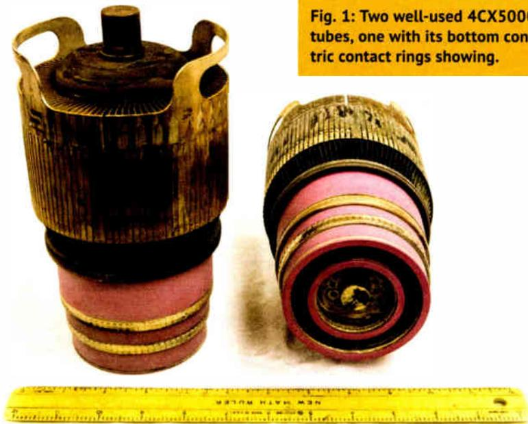
Fig. 1: Two well-used 4CX5000A tubes, one with its bottom concentric contact rings showing.
