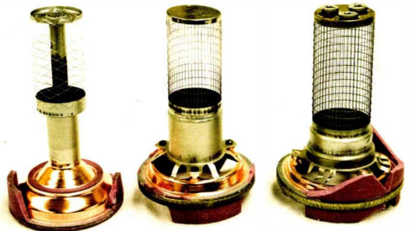
Fig. 4: Filament, control grid and screen grid, from left.
