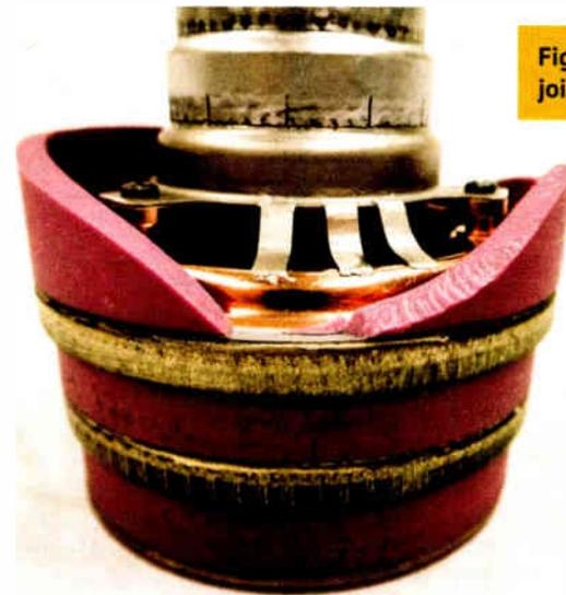
Fig. 3: A screen grid joined to a contact ring.
