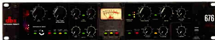
The dbx 676 uses a high-gain, Class A tube preamp section based around a 12AU7 vacuum tube that can be adjusted to either sound clean or dirty and full of harmonic character. The 676 uses the compressor/limiter design from the dbx162SL along with a three-band parametric EQ. It adds a post-tube attenuation control.
