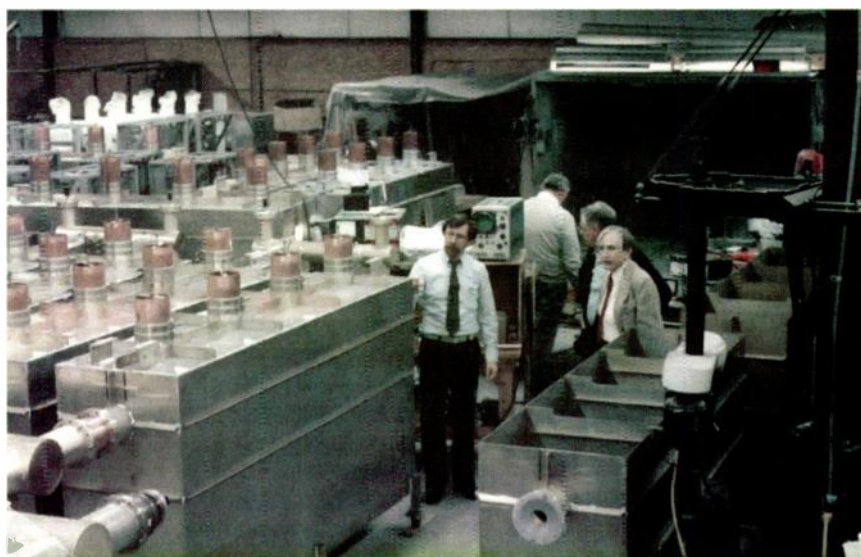
Left: On the shop floor at Shively Labs in 1984, Bob Surette, left, and Ed Shively, far right, inspect cavities destined for the 441 site, a multi-channel tower facility built by Guy Gannett Communications in the Miami area. The combiner was the first band-pass filter system that used square cavities and group delay equalizers in the United States, Surette said.
