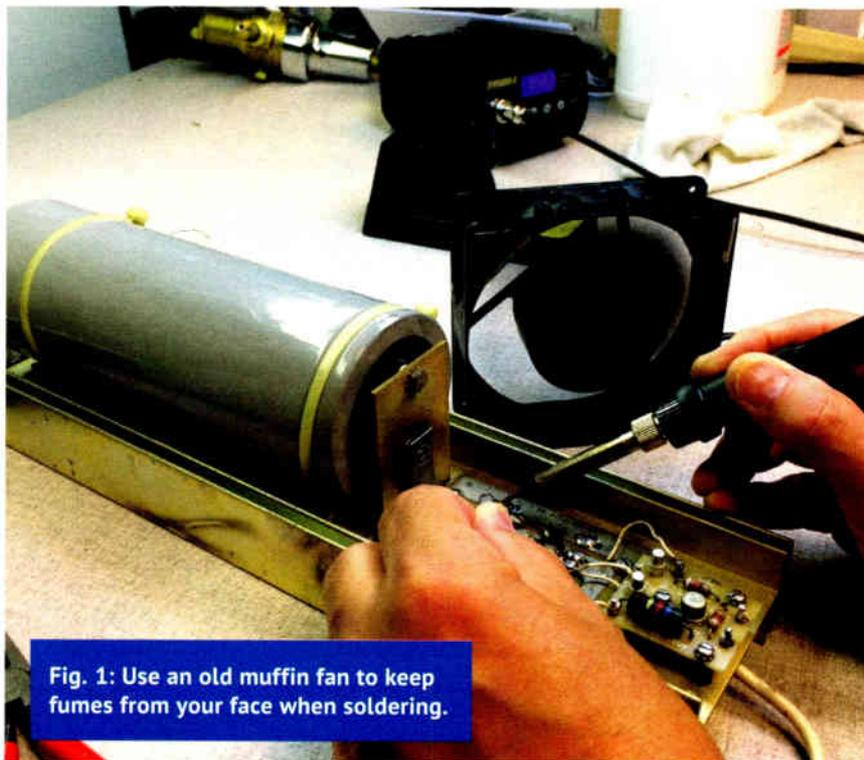
Fig. 1: Use an old muffin fan to keep fumes from your face when soldering.
