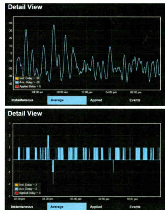
Barber said correct time alignment can take a station (top image) from \pm 36 samples to \pm 2 samples.
