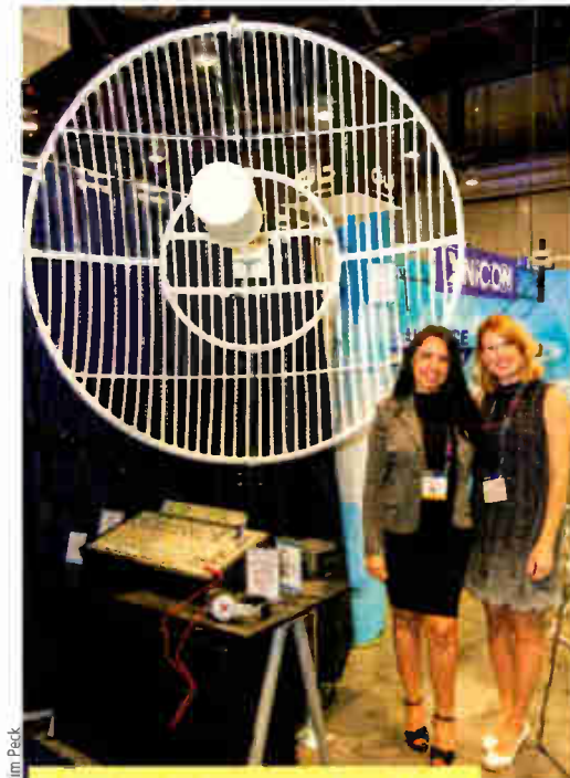
Andrea Zambrano and Shannon Piagentini show off a Nicom 8-foot grid antenna for 950 MHz use.
