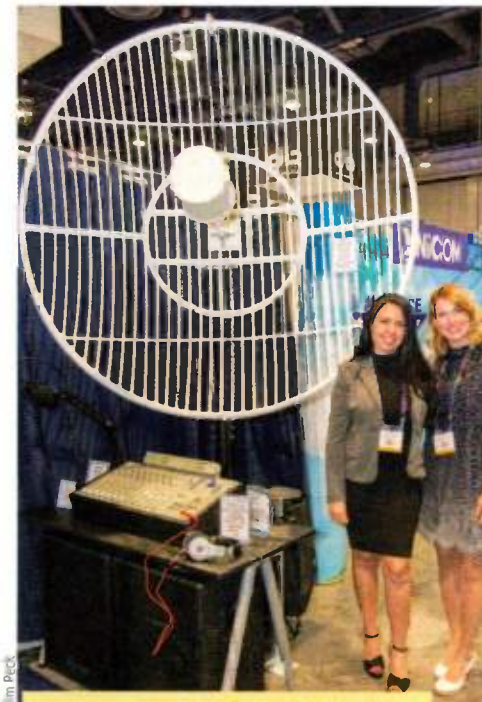
Andrea Zambrano and Shannon Piagentini show off a Nicom 8-foot grid antenna for 950 MHz use.
