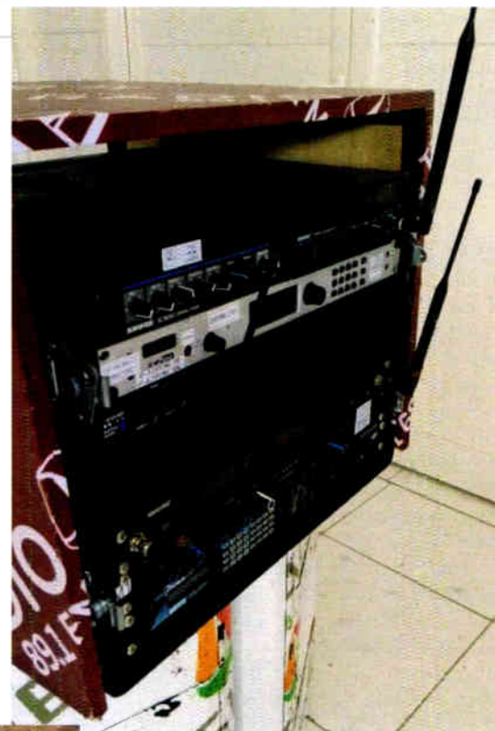
The equipment rack with the Telos Z/IP One in the center.
