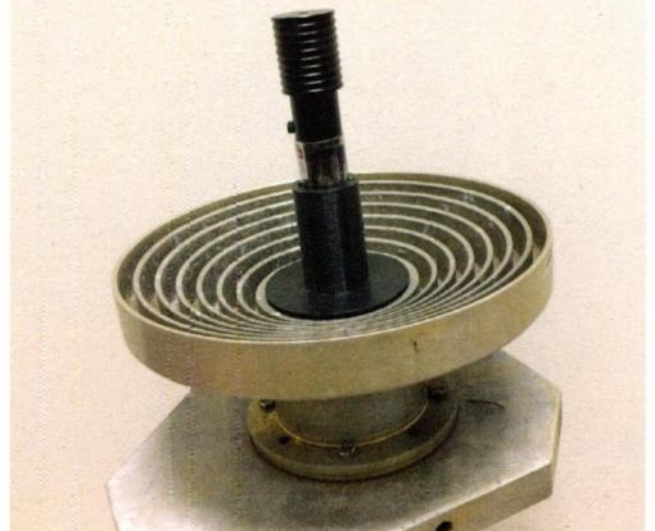
Fig. 4: The laser pointer fits inside. The laser should point directly to the center of the dish. If not, the feed horn mount can be adjusted.
