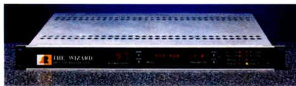
In addition to monitoring standard AM modulation, the AMMA-2 monitors modulation-dependent carrier level AM transmissions.
