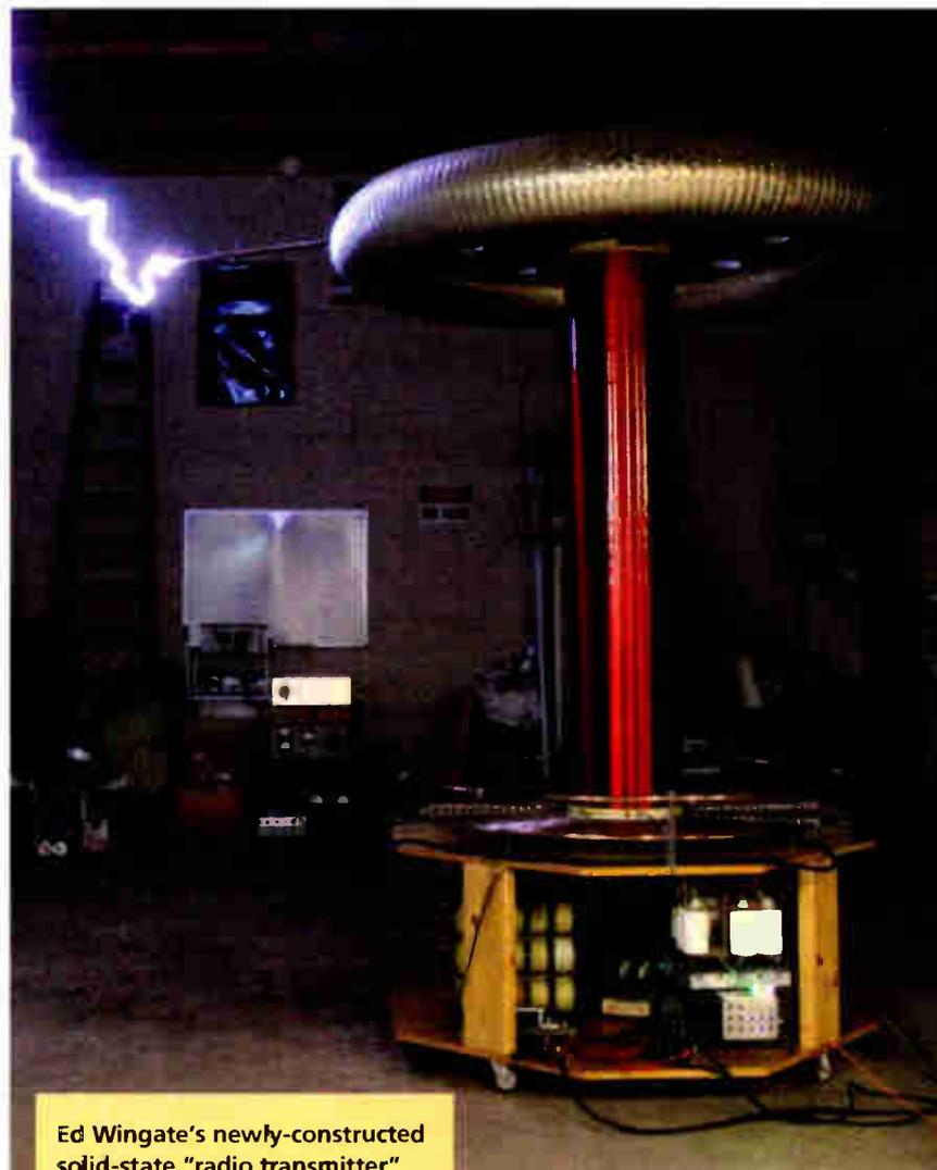
Ed Wingate's newly-constructed solid-state "radio transmitter" is designed to radiate most of its output in the form of corona discharges.
