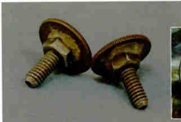
Fig. 3: The flip side shows the discs glued to the bolt top with heavy-duty epoxy.
