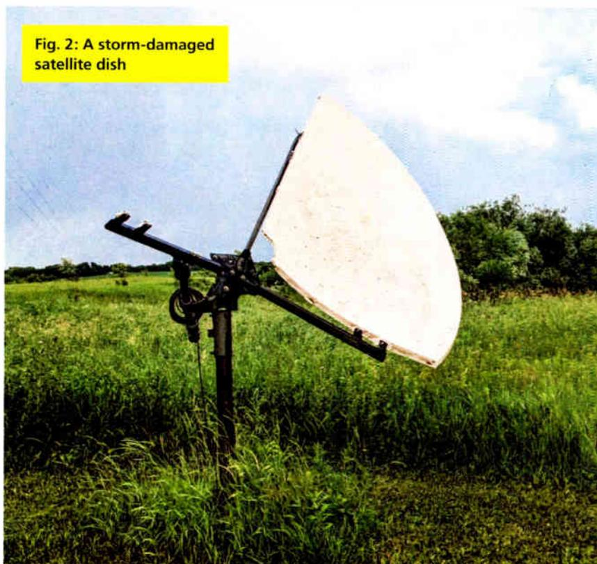
Fig. 2: A storm-damaged satellite dish
