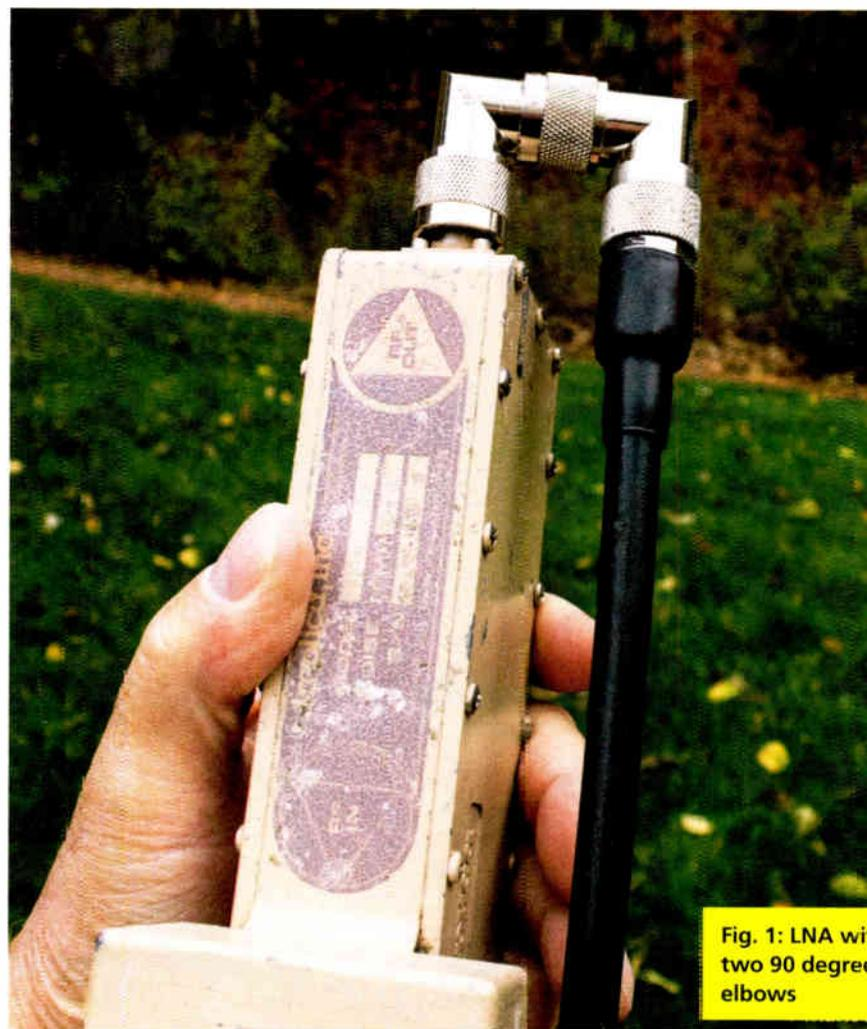
Fig. 1: LNA with two 90 degree elbows
