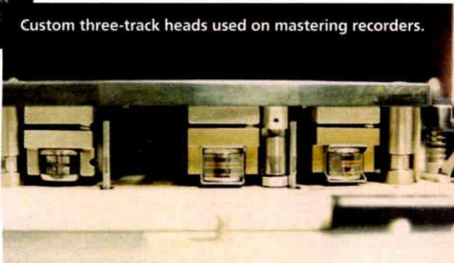
Custom three-track heads used on mastering recorders.
