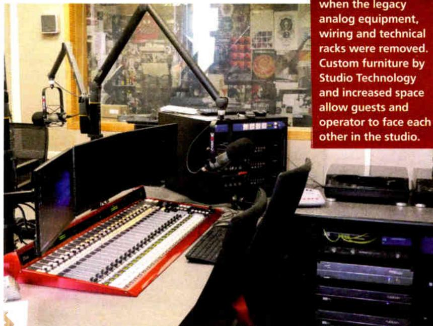
The WRSU Air Studio was reconfigured when the legacy analog equipment, wiring and technical racks were removed. Custom furniture by Studio Technology and increased space allow guests and operator to face each other in the studio.
