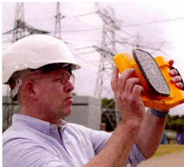
Left European electricity transmission system company TenneT used a Fluke ii910 Precision Acoustic Imager to troubleshoot an interference problem at an airport.
