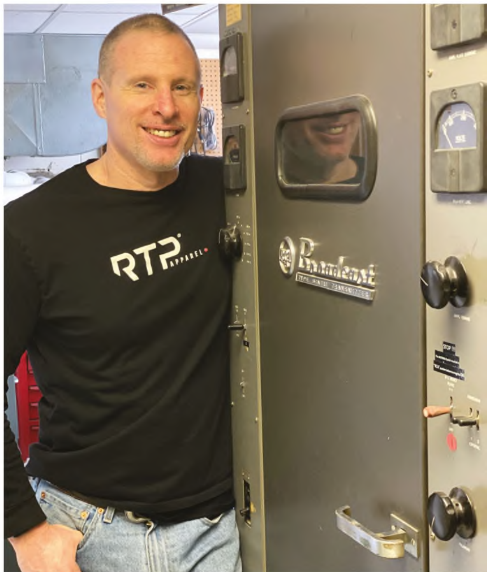
Above Brian Walker with the 1963 RCA vacuum tube AM transmitter that was used when WBTC(AM) in Uhrichsville, Ohio, went on the air. It is still operational and used as a backup.
