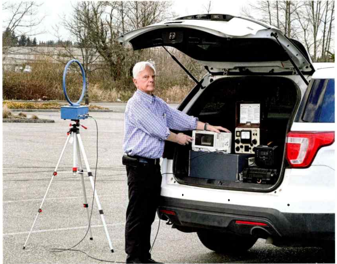
Above Jim Dalke is shown at a station site, preparing to make its field measurements. The field meter next to the spectrum analyzer is used to check harmonics.
