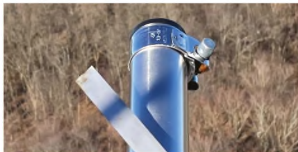
Left The ribbon suffered bending fatigue and broke near the mount.
