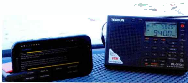
Above An example of receiving text via shortwave. An Android device with the necessary app sits next to a portable shortwave radio. No patch cord.
