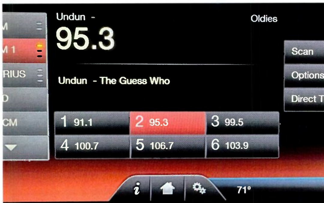
Above In my unconnected car's entertainment system display, RT is displayed in the center. DPS info is displayed at the top right above the frequency and it scrolls, and it is also displayed on an aux screen in the instrument cluster.
