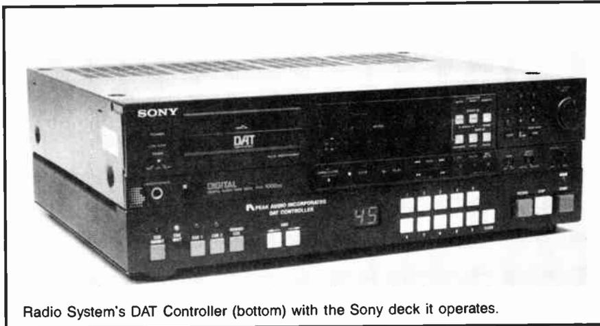
Radio System's DAT Controller (bottom) with the Sony deck it operates.
