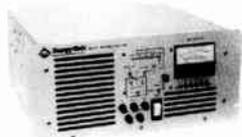
Amplifiers and transmitters are available at the popular levels of 25, 100, 300, 500, 1000, 1500, 2000, 2500, 3000, 4000 and 4500 watts. All units are broadbanded and designed for local and remote operation.
