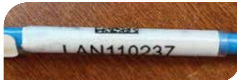
Fig. 3. A test label with 2D code and wire number.
