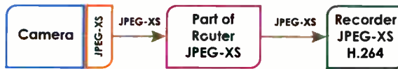
Ideal: All Devices Use I/O 1.5Gb JPEG-XS Using 4K JPEG-XS with a router
